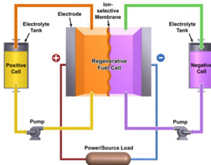
*Diagram: a Redox Flow Battery*
