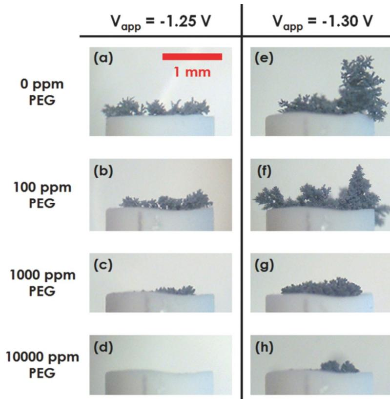
*Formation of these needle-like zinc dendrites from repeat electrodeposition can cause a problem with zinc flow batteries, requiring periodic stripping. Such electrochemical side effects happen frequently with complex battery chemistries, but may be predicted and mitigated through careful research, modeling and design. Photo Credit: Stephen J. Banik and Rohan Akolkar, Department of Chemical Engineering, Case Western Reserve University.*
